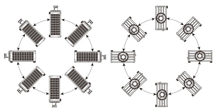
You can change the direction of the image using the Projection Mode. The projector has a smart cooling mechanism, which regulates the fan automatically according to the projection mode.
