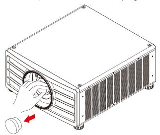
2. Push the lens into the lens mounting hole and turn it clockwise to the "Lock" position. When turning the lens, the "Click" sound indicates that the lens is completely fixed and locked in place.
