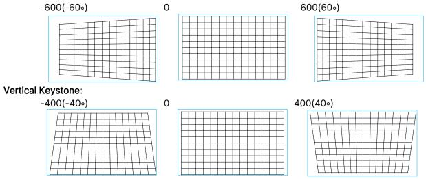
Besides correcting H and V Keystone by separate, you can use H and V keystone combination to correct the distortion. In this case, the effective range may be limited.
