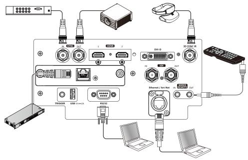
HDBaseT/LAN (Network control): The projector supports network control. LAN and HDBaseT share the same port. If only network control is used, you can connect the LAN on the projector to PC or through the local network. Refer to the Remote Communication Manual for detailed information.
