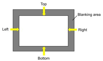
**Top:** Press the the  $\triangle$  or  $\nabla$  button to adjust the top blanking area on the projected picture.
