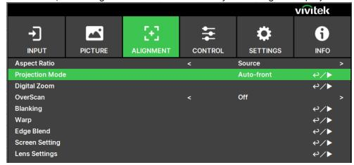
Use the  $\triangleleft$  or  $\triangleright$  button to select a projection mode to flip the projected image as installation orientation or viewing direction. The selection options are described as below.
