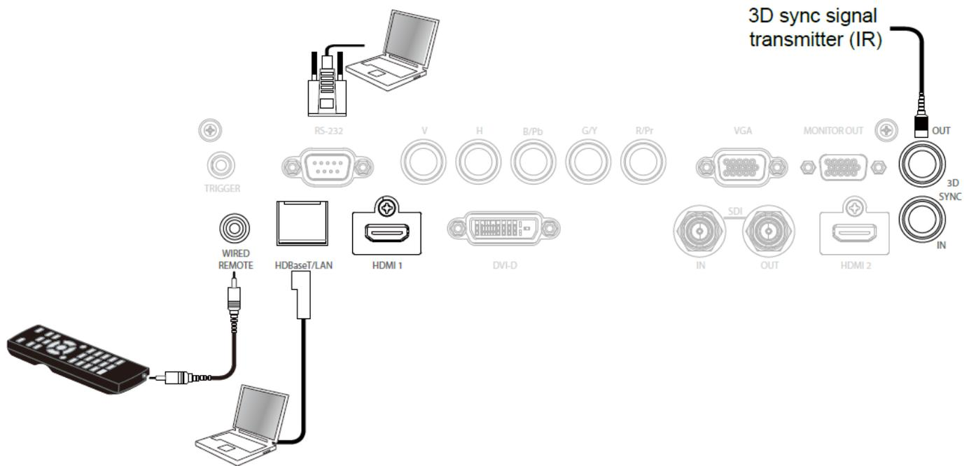
**HDBaseT/LAN (Network control):** The projector supports network control. LAN and HDBaseT share the one port. If only network control is used, you can connect the LAN on the projector to PC or through the local network. Refer to the Remote Communication Manual for detailed information.
