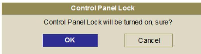
Once Control Panel Lock is enabled, all of control buttons on the projector are locked. Below message is shown on the screen few seconds if any control buttons is pressed.
