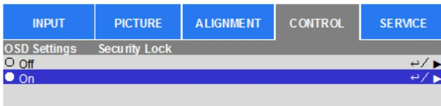
Once Security Lock is turned on, the pop-up message for setting up the password Lock as is shown as below. Press arrow buttons to set up your password, the password can be the combination of four arrow keys.
