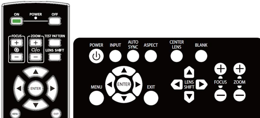
1. To open the OSD, press the **Menu** button on the OSD control panel or remote control. There are five folders on the menu. Press the cursor ◀ or ▶ buttons to move through secondary menus.
