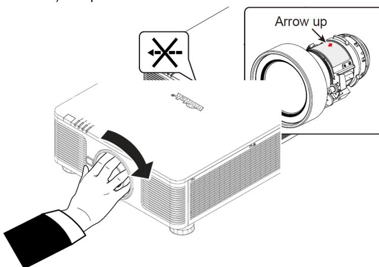
3. Make sure the lens is pushed into the holder and turn it clockwise to the "Lock" position. When turning the lens, the "Click" sounds twice to indicate that the lens is completely fixed.
