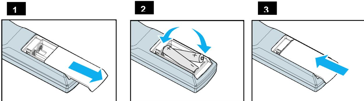
1. Remove the battery compartment cover by sliding the cover in the direction of the arrow.
